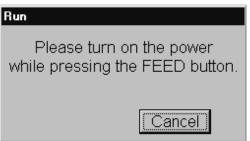
**3.** At this time, connect the printer to the PC with the RS-232C cable. Press and hold the FEED button while sliding the printer Stand-by switch to ON. When the printer enters DOWNLOAD mode successfully, the message screen will change to the following.
